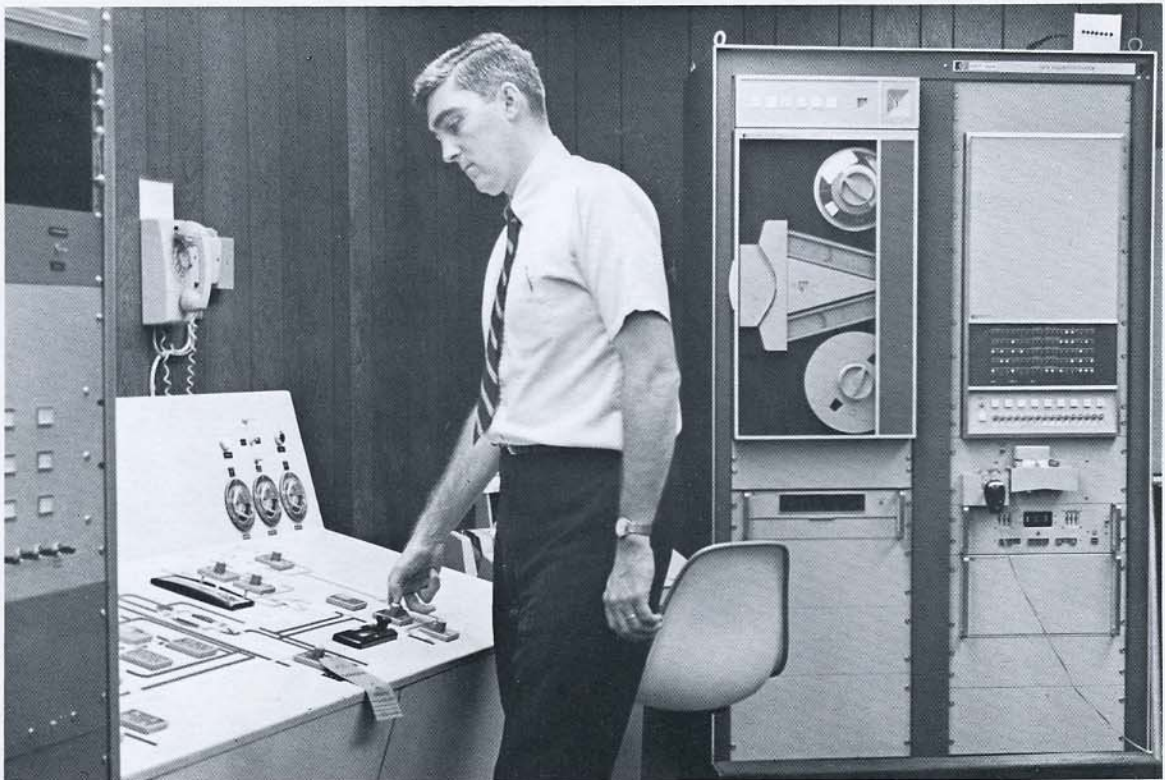
The computer-controlled digital data acquisition system (right) and control console are located in a control room overlooking the test area (photo on rear page).
